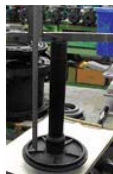
B2 : The length of the shaft sleeve from the tip of the shaft sleeve to the top of one of the radial ribs.
