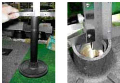
B1 : The length of the shaft sleeve from the tip of the shaft sleeve to the top edge of metal threading inside the impeller.
